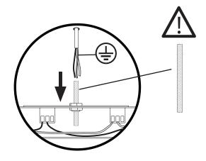
Insert anti-abrasive heat sleeve before making your connection.
