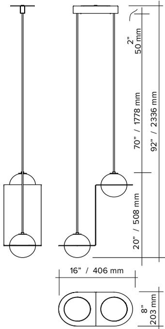
parallel wires with offset connection
