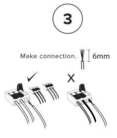
Ensure no wires are scratched or pinched during this operation.
