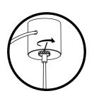
Adjust the height of your cable hangers (**X**) by lowering or raising the aircraft cable. Losen lock ring, adjust cables, then retighten lock ring.
