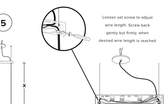
Trim wires to desired length (X). Do not leave a large excess of wires inside canopy. Reconnect them as before.
