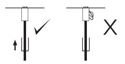
Ensure no wires are clipped or pinched during this operation.
