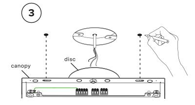
Before marking your anchor points, align the ceiling disc with the center of your junction box. Use canopy as a guide.
