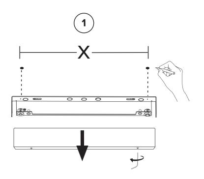
Lower ceiling bracket cover then use the bracket as a guide for your anchor holes. Make sure to use appropriate anchors for ceiling material.
