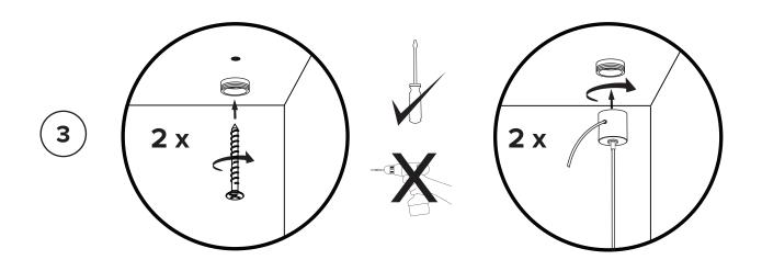
Make sure you use appropriate anchors and screws for your ceiling material and luminaire weight.
