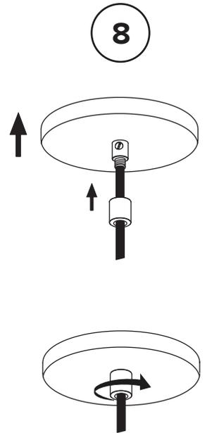
Ensure no wires are clipped or pinched during this operation.
