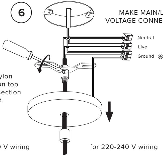
Tighten nylon set screw on top of sleeved section of cord.
