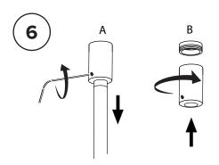
Loosen set screw and lower celing rod to allow mount to be screwed into the ceiling anchor
