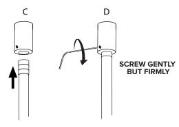
Raise ceiling stems into the anchored ceiling mount and tighten the set screw
