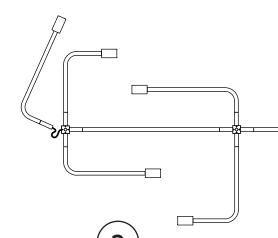
Insert removed arms into the cubes and secure set screws. The arms will be repositioned properly once the fixture has been installed to the ceiling.
