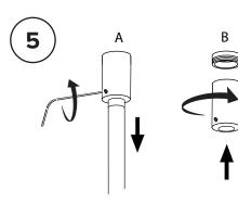
Loosen set screw and lower celing rod to allow mount to be screwed into the ceiling anchor
