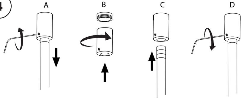
Loosen set screw and lower ceiling rod to allow mount to be screwed into the ceiling anchor
