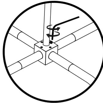
Losen set screw, reposition arm then tighten set screw gently, but firmly.
