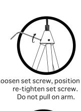
Loosen set screw, position arm, re-tighten set screw. Do not pull on arm.
