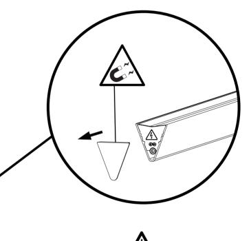
Becareful when removing endcap that it does not stick to other surfaces which could result in scratches in the paint. The adjustment screw holding the balance weight is now visible. Use supplied allen key to screw weight in or out depending on balance.
