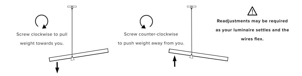
The adjustment screw holding the balance weight is now visible. Use supplied allen key to screw weight in or out depending on balance.
