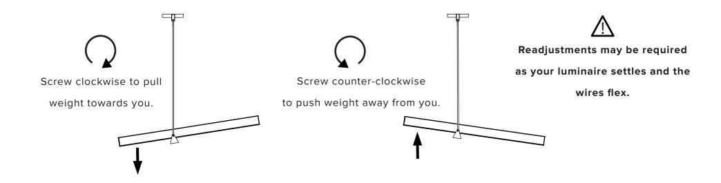
The adjustment screw holding the balance weight is now visible.
