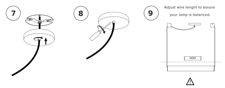
Readjustments may be required as your luminaire settles and the wires flex.
