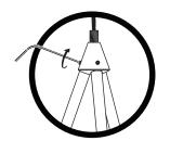
Loosen set screw, position arm, re-tighten set screw. Do not pull on arm.
