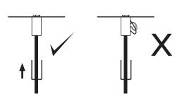
Ensure no wires are clipped or pinched during this operation.
