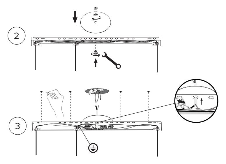
Before marking your anchor locations, align the ceiling bracket with the center of your junction box.
