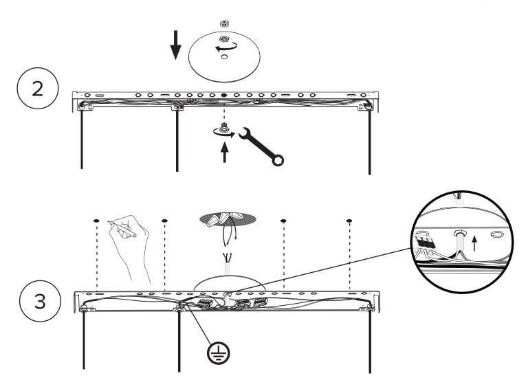
Before marking your anchor locations, align the ceiling bracket with the center of your junction box. Make sure to use appropriate anchors for ceiling material.
