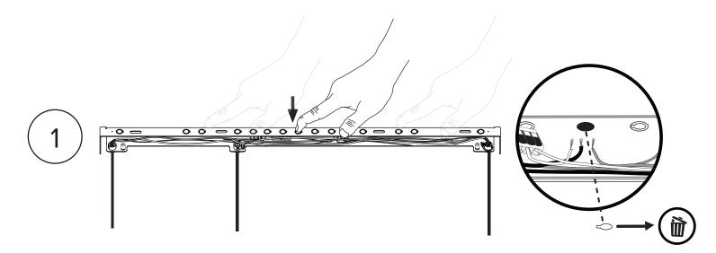
Knockout selected hole depending on desired electrical box alignment.
