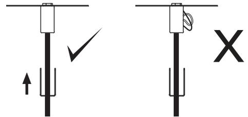
Ensure no wires are clipped or pinched during this operation.
