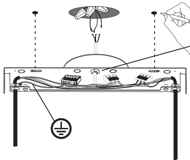
Before marking your anchor locations, align the ceiling bracket with the center of your junction box.
