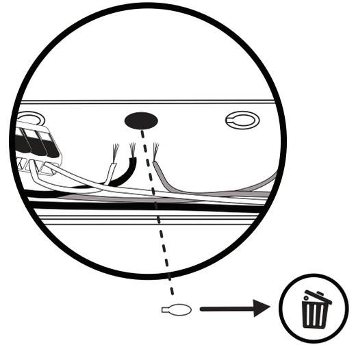
Knockout selected hole depending on desired electrical box alignment.
