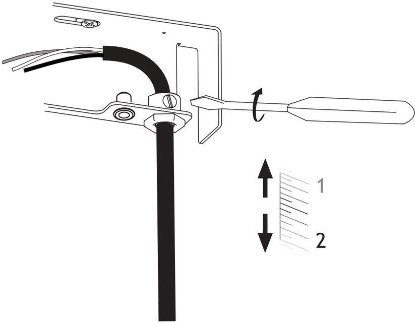
Make sure the globes are level by micro-adjusting the wire lengths.
