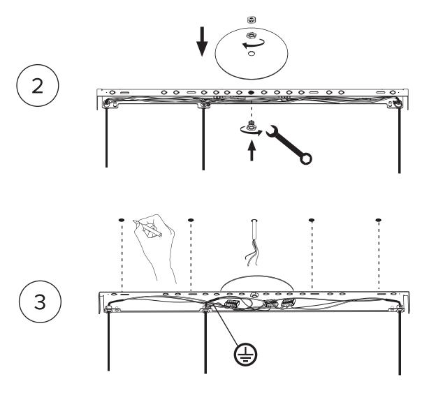
Before marking your anchor locations, align the ceiling bracket with the center of your junction box.
