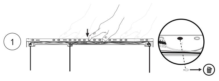
Knockout selected hole depending on desired electrical box alignment.
