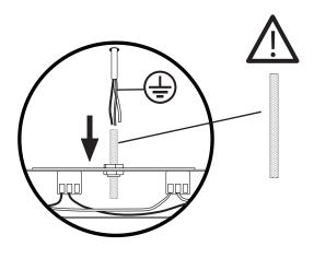
Insert anti-abrasive heat sleeve before making your connection.
