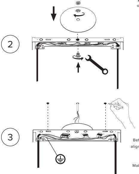
Before marking your anchor locations, align the ceiling bracket with the center of your junction box.
