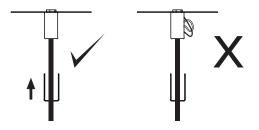
Ensure no wires are clipped or pinched during this operation.
