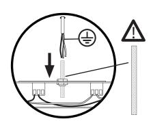
Insert white anti-abrasive heat sleeve before making your connection.
