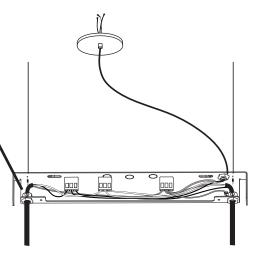
Trim wires to desired length (X). Do not leave a large excess of wires inside canopy. Reconnect them as before.
