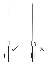
Ensure no wires are clipped or pinched during this operation.
