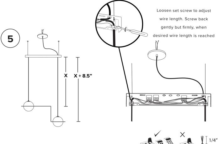
Trim wires to desired length (X). Do not leave a large excess of wires inside canopy. Reconnect them as before.
