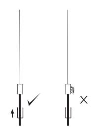
Ensure no wires are clipped or pinched during this operation.
