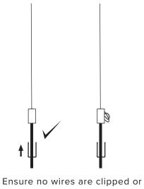
Ensure no wires are clipped or pinched during this operation.
