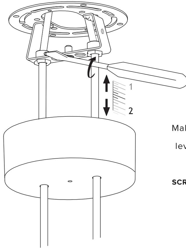
Make sure the globes are level by micro-adjusting the wire lengths.
