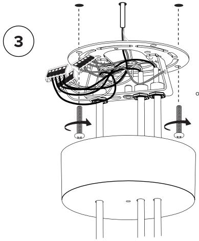
Ensure no wires are scratched or pinched during this operation.
