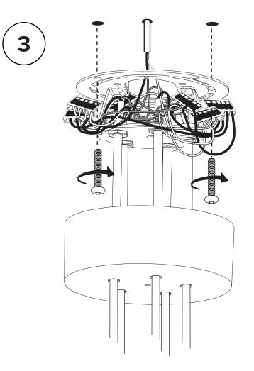
Ensure no wires are scratched or pinched during this operation.
