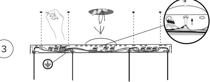
Before marking your anchor locations, align the ceiling bracket with the center of your junction box. Feed wires through anti-abrasive sleeve before making connection
