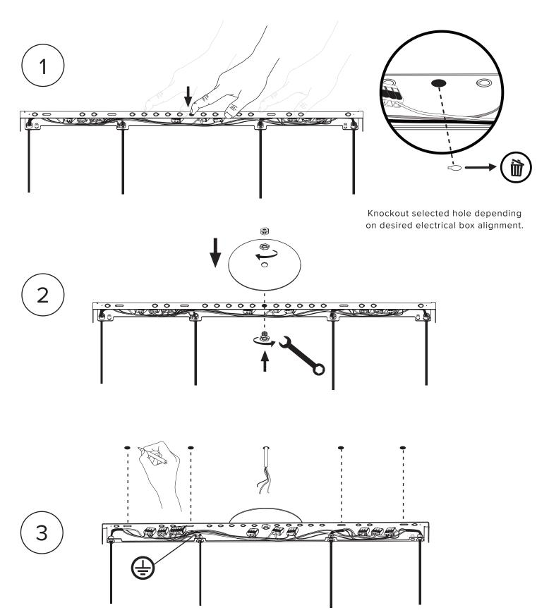
Before marking your anchor locations, align the ceiling bracket with the center of your junction box.
