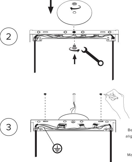
Before marking your anchor locations, align the ceiling bracket with the center of your junction box.
