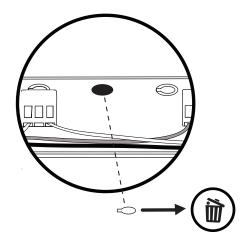
Knockout selected hole depending on desired electrical box alignment.
