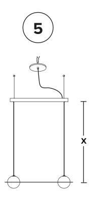
Loosen set screw to adjust wire length. Screw back gently but firmly, when desired wire length is reached
