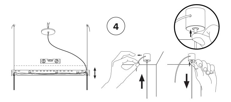
5 5 × Loosen set screw to adjust wire length. Screw back gently but firmly, when desired wire length is reached
