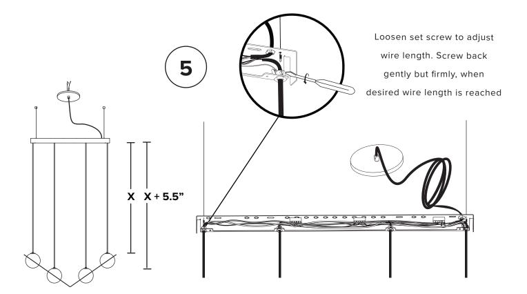
Trim wires to desired length (X). Do not leave a large excess of wires inside canopy. Reconnect them as before.
