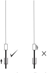
Ensure no wires are clipped or pinched during this operation.
