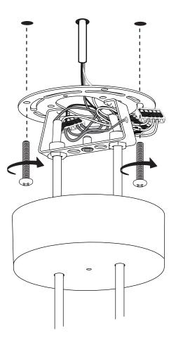
Ensure no wires are scratched or pinched during this operation.
