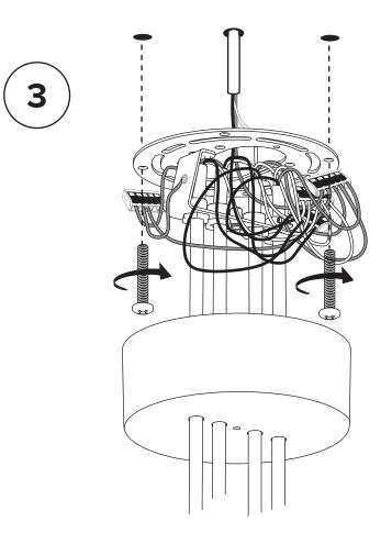
Ensure no wires are scratched or pinched during this operation.
