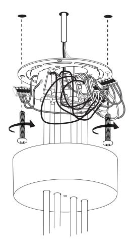
Ensure no wires are scratched or pinched during this operation.
