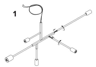
Rotate each arm 5 full rotations counterclockwise before inserting arms into body to prevent wires from over twisting.
